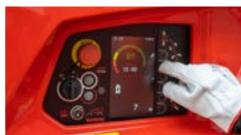
The large screen at the lower control box offers additional information to the top control box for operator and allows technicians to carry out a quick diagnosis, consult the machine memory and many other functions.
