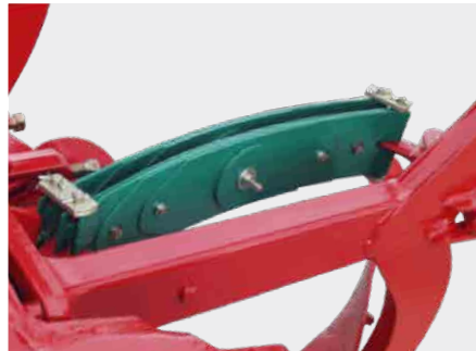
Double spring package with 14 leaves (1400 kp)
