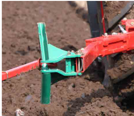
Packer arm connecting to the packer
